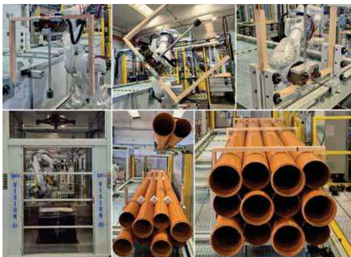
Automatic packaging and palletising system equipped with robots and artificial intelligence
