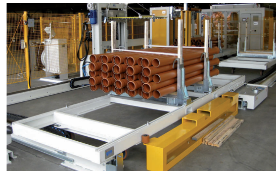
An IPM plant for packaging and palletizing pipes
