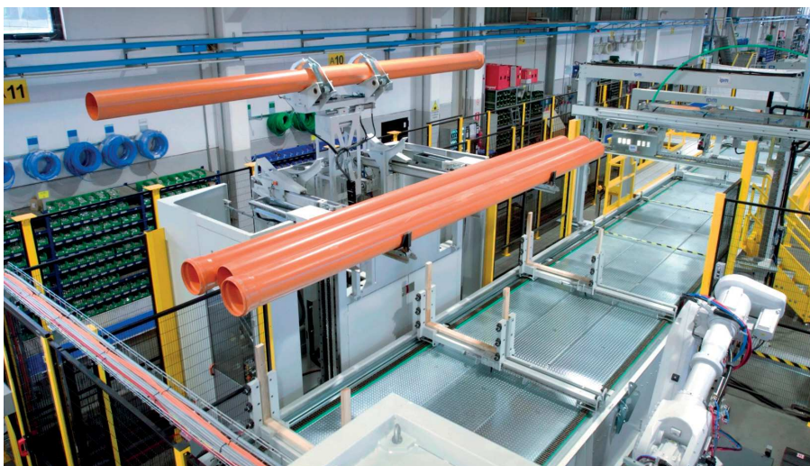
System for forming pipe pallets with opposing ends.
