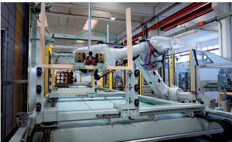
Robot in action positioning wooden frames for the production of pipe pallets on an IPM line.
