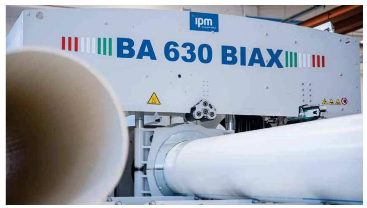
What is PVC-O? PVC is a polymer whose molecules oriented at random. In PVC-O, under certain conditions of pressure-temperature-velocity, stretching the material results into the ordering of the molecules, thus forming a laminar (layered) structure that significantly improves the physical and mechanical properties of PVC, providing exceptional characteristics and additional extraordinary competitive advantages, while maintaining the characteristics of the raw material of origin.
